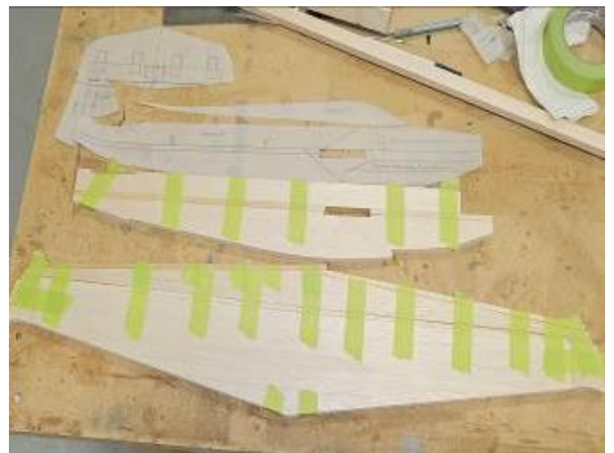
Here's the initial fuselage & wing Lay up. Note the Full Length hardwood Spars on both fuselage & wing.
