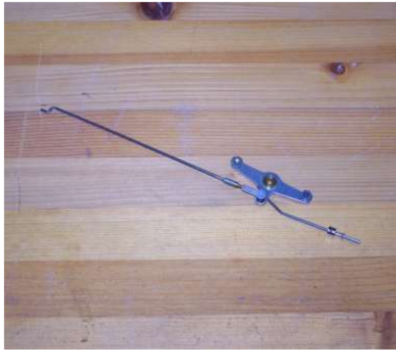
Figure 5. Using an outboard bellcrank mounted under the wing requires the pushrod linkage to look something like this. The collar is used to adjust the trip position relative to the elevator for the sensitivity your pilot likes. A washer soldered to a bit of tubing makes up the "pusher" that contacts the trip wire. The collar is a bit too big to fit in the small space between the shutoff and the fuselage. The wire is trimmed so it just clears the engine case at full down elevator.
