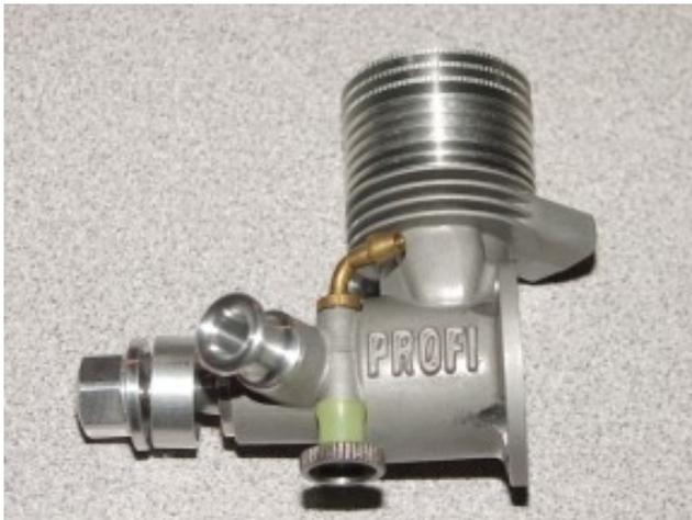
With head space set at .005" and my 31K test prop it blew away my previous 34K rpm numbers. With 30% nitro it went 36,000! It blew the plug totally on two runs. Back to 15% nitro, same head space rpm was 35,380! On 15% the plug looks new after 3 runs. It almost sounded like there was no change between 15 and 30% nitro. I took the prop back to my VAMkII which had turned it at 31K and got 31,020 rpm, no change (this was 15% as my VA doesn't like anything more than 20% the way it is setup).
