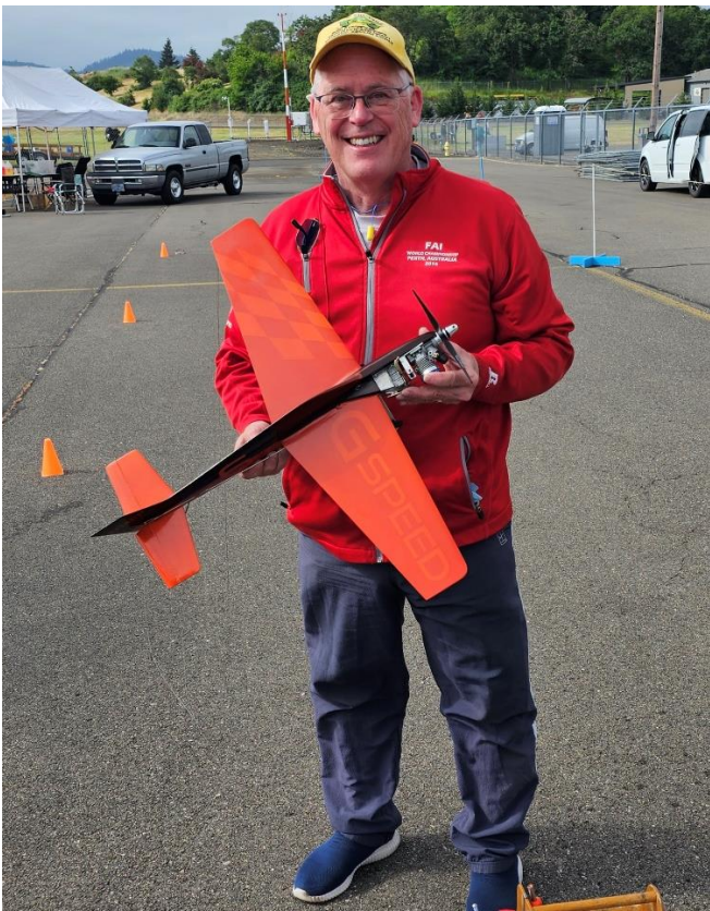
Paul Gibeault and his new Polecat Scale Race model. Built from a modified Pat King LLC laser cut kit. Magnum XLT .15 motor with Bill Bischoff tank, shut off & landing gear.
