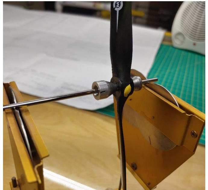
Don't you believe it! The Prop needs this amount of hub weight to balance properly. Balance is easily checked with a bit of plasticine.
