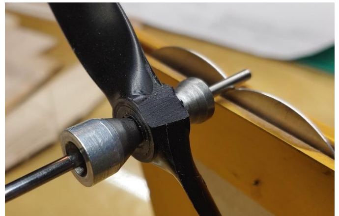
Weight removed from opposite side gives the desired effect. Prop now balances 360 degrees in all directions. Winners are often skeptical about manufacturers claims... It's attention to details like this that can put you ahead of the competition.
