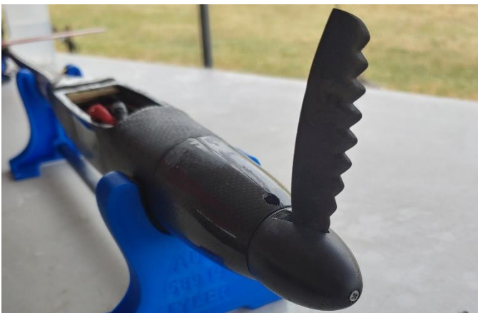
Wanna go really fast? If you don't have prop restrictions maybe go for a L/H shark tooth monoblade prop. Complete with 3D printed spinner.
