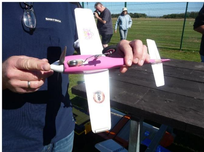
Here's the underside of Jon's Odeyn's winning racer. In addition to using a Cox 290 motor with separate tank, he used a coil spring landing gear and metal nose skid. Jon's fuselage strength was much improved over the stock plan version. Very effective over grass.
