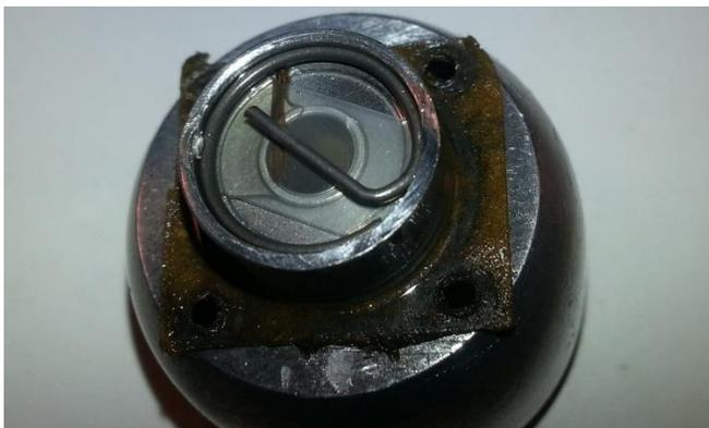
And of course, they really run quite well up until the time the piston separates! This situation was caused by my negligence in not checking the ball-socket joint play prior to racing. I lulled myself into thinking that using their lower 30% nitro fuel, a loose ball-socket was not likely to be a problem.
