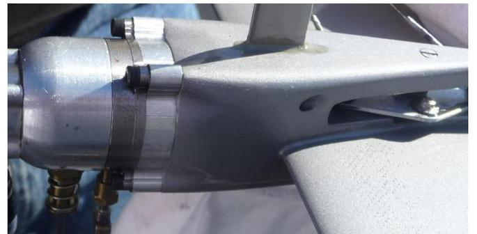
**Note venturi air hole in fuselage just ahead of the bellcrank slot.**
