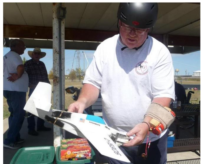
To the victor the spoils & to the unfortunates... the trash bin. Les Akre's Gillott Rossi powered L'il Mike G/Y model hit the pavement hard when his up line broke in level flight. OUCH!!
