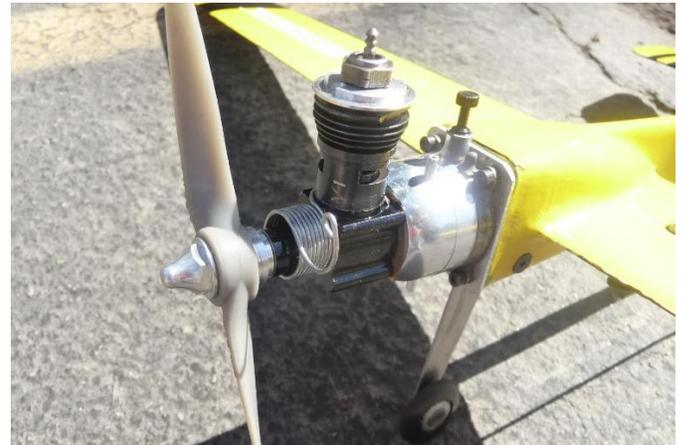
The business end of The Gibeault "Streaker V" entry. \*Note the Doug Galbraith head fitted with a Nelson glow plug that costs half the price of a Cox glow head. This Cox Venom uses a stock Cox 5-40 stud screw & Cox spinner to avoid crankshaft shearing & sheet L.G for improved drag reduction.
