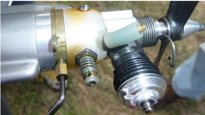
Note in the upper photo, John's faired in bellcrank assembly & very clean landing gear installation. Bottom pic is a view of John's tank which features a fine thread locking collet NVA, mechanical overflow valve, & unflow vent pipe for very stable inflight running. Note that John runs the original Cox TeeDee glowhead & his own prop.
