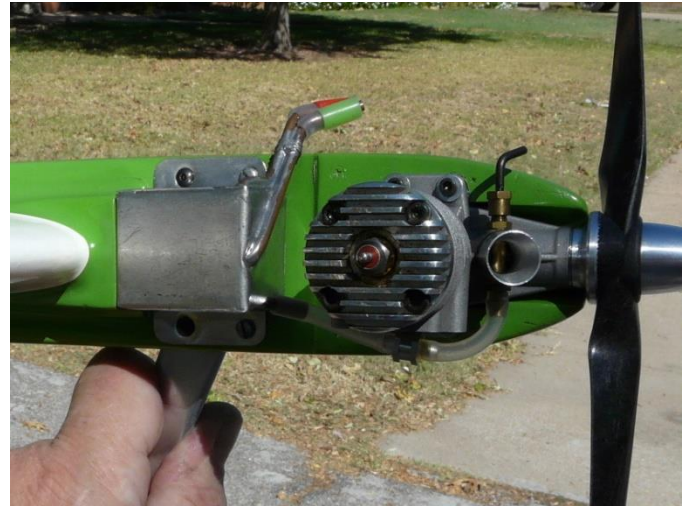
The Finished Fuel Tank Mounted On a "Mockingbird" SSR.
