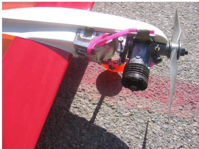
The Business end of Doug Mayer's New "Retro Baby" Fox Racer. Note the Generous Cheek Cowl to absorb the Fox .35's inevitable vibration.
