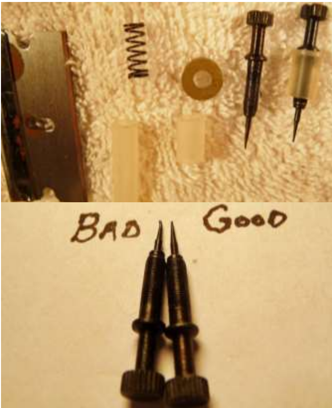
(Top), needles showing the tubing seal mods, (bottom) damaged, and good needle tips.
