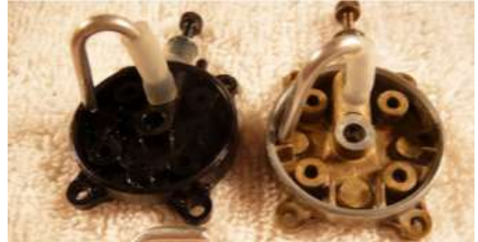
The replacement pick up tube is bent from 3/32" O.D. soft aluminium tubing & chamfered at the bottom to fix exactly. Silicone tubing attaches it to the tank back.
