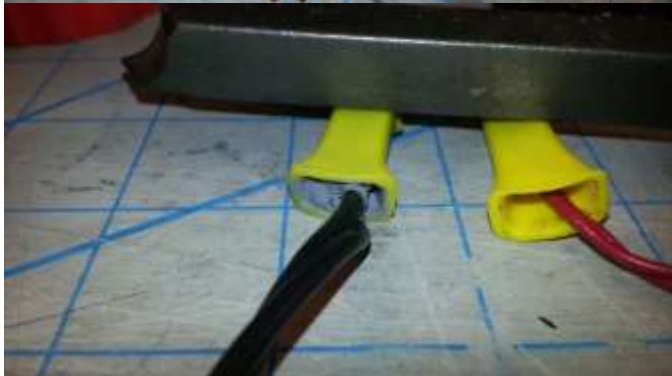
Cox Clip fitted with larger, low resistance wire, then sealed with RTV produced much better glow with less power.
