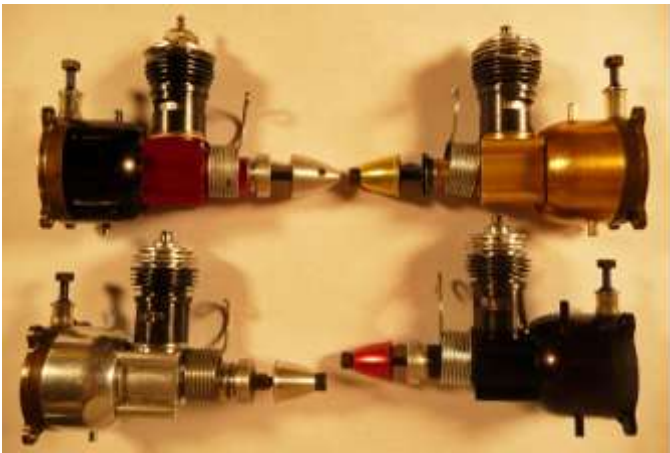
Cox .049 mouse racing engine variants: Top L-R: Venom w/ Galbreath head & Golden Bee. Bottom L-R: Silver Bee & Black Widow.
