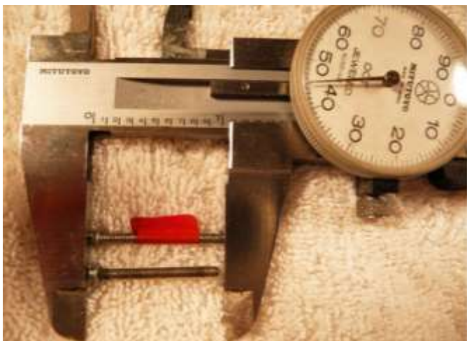
This example is over .100" longer than Standard! Too long and the tank won't seal.
