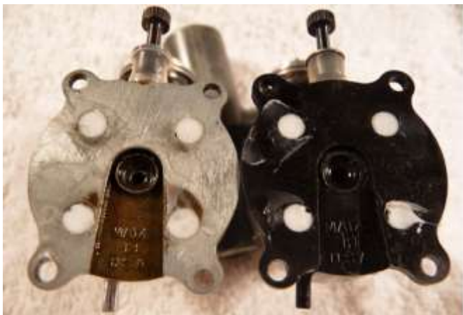
After final assembly, the tank screw hole areas are filled with RTV silicone sealant for leak prevention.
