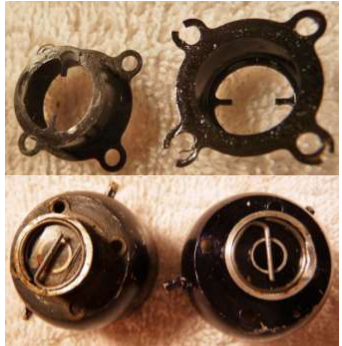
Black Widow tanks: note severe wear around reed flange holes on reed retainer(Top) excessive wear on top of reed retainer (Bottom) cracked retaining "G-Clip area and reed seal vent hole area.
