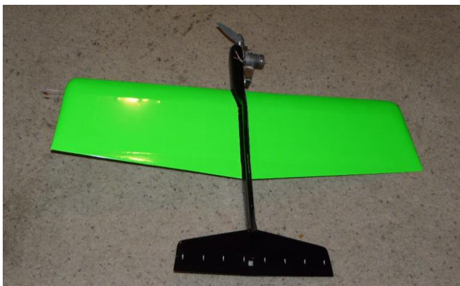
Bill Bischoff's modified Brodak Super Fly. Wing is shorter with increased Chord width. Ask Bill For details.
