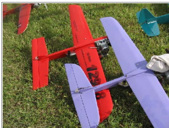
“Muffler” Rats – TQR with Jett 30 and muffler. Venturi restricted to approximate TQR speeds
