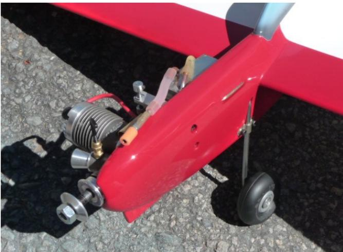
Mono-wheel gear is a new SCAR rule to ease "turn-in" problems with two wheel gears. Ron used oversized wire for reliability. The "depth" of the canopy achieved by the paint shading technique is remarkable.
