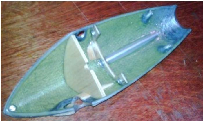
We can adjust the heat of the air to the engine in several stages from full hot to full cold. All the passage-ways are visible in the photos along with some of the plug/restrictors to control the flows.”
