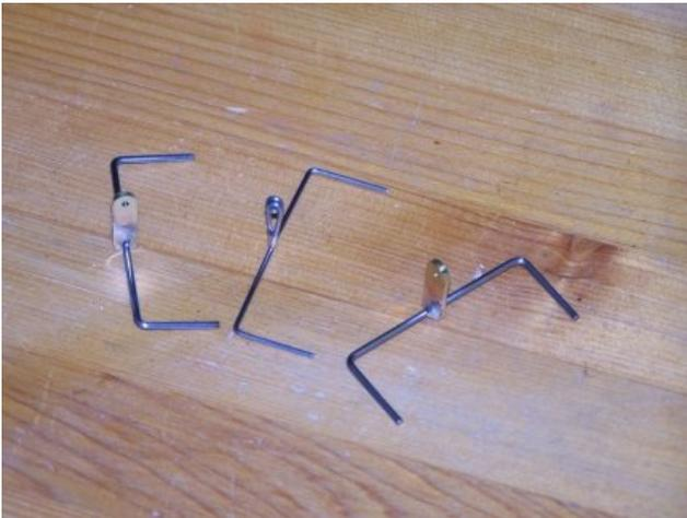
Figure 1. (3838) Three elevator horns were made to check out the possibilities. The quickest to make is the formed wire unit in the center. Only one part is required, not counting the wire wrap. This one was bent around a 1/16" pin forming the hole for the pushrod. It was then wrapped with .007" copper wire and soldered. The other two units are made from 1/16" music wire and .062 brass stock arms and silver soldered together. Close fits and big fillets used to improve strength.
