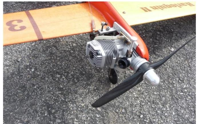
A close up of Jed Kusik's OS .35 AX powered Rat. Custom venturi, Dirty Dale shutoff(?), OS needle, conformal vent fitting, carbon APC prop(?) and looks like new! (Photo: via Ron Duly)
