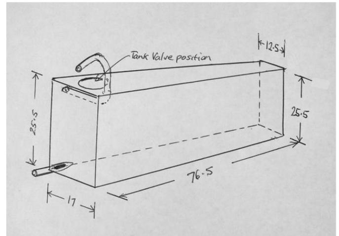
After making the template, marking the tin and cutting out the shape, it is simply bent around the block (use softer 'round' bends rather than hard hammered right angles) and the longitudinal seam is soldered with the block inside. A 3 mm overlap is all that is needed. Include that in your pattern. The block is then gently tapped out and your tank is well on the way to being finished. The tinplate used measures 0.25 mm. Nice and easy to bend around the block.
