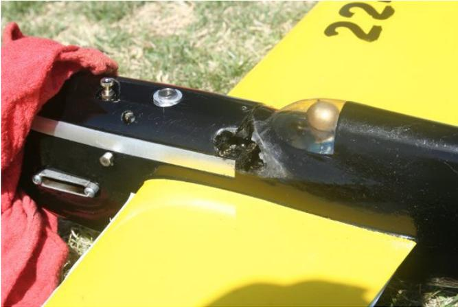
Cockpit full of fire damage and a hole burned through the cowl.
