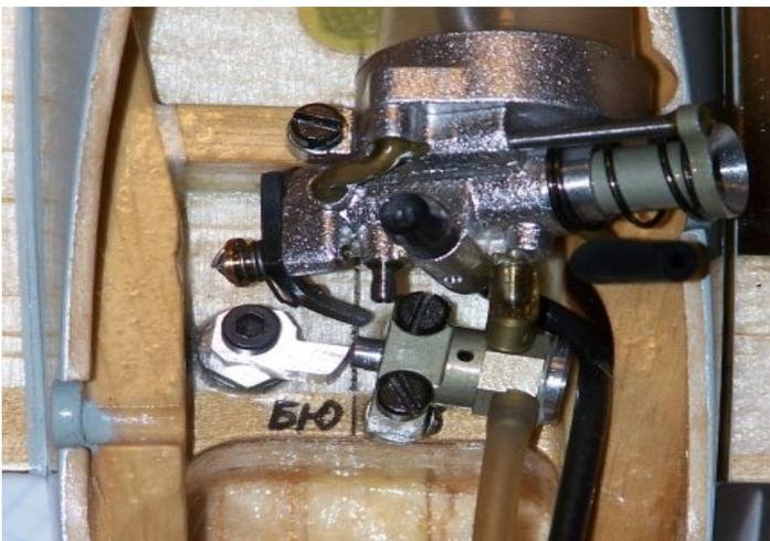
Changing the shutoff arm to a shorter, thicker design eliminates the interference with the regulator, but still makes adequate contact with the tank shutoff lever. Hopefully, the contact geometry (not great) does not result in excessive contact forces that will wear the arm and compromise the system. With this setup, the pilot can wiggle his hand with satisfying results. (Photo: Hull)
