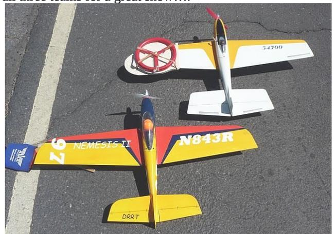
Ron and Don's B T/R planes. Ron's is a close copy of Don's original Nemesis. Note the external refueling tube. Not as prone to fires as a valve on top of the fuselage (but not totally immune) due to over-prime.
