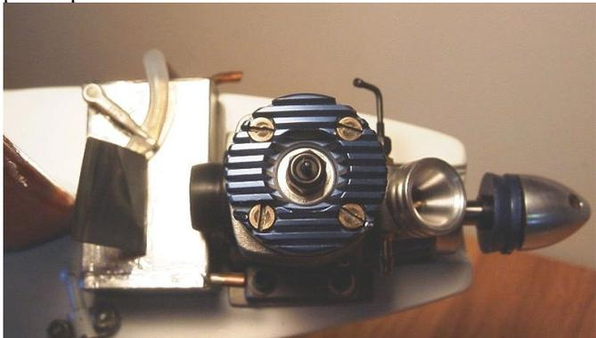
Here it is shown with motor, a Novarossi CX .15. There is no room for a shutoff with this setup, and barely room to squeeze in a fuel filter!
