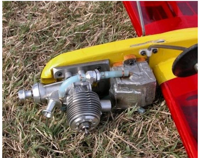
Bottom view shows fuel pickup tube location at the widest part of tank & at the very bottom. Little details like wiring on the fuel lines can help prevent ruining your day!
