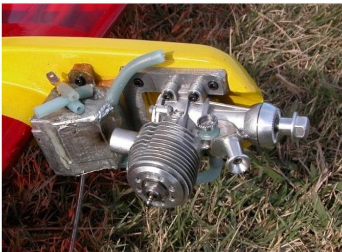
Thanks to Bill Lee for these photos of Russ Green's Fora .15 powered Clown. This F2D Combat engine makes major power in spite of the tiny 4MM venturi. Russ reports airspeed of 17.9 seconds & mileage of 42 laps per tank. No shutoff, notice the cushioned alligator clip overflow pinch off.
