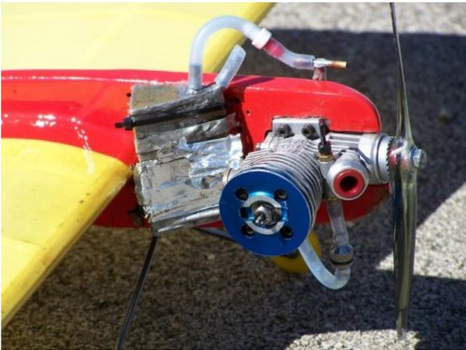
Al Ferarros' 2006 Nats winner is a model of simplicity. He always seems to place well with this rig. Motor is an O.S. TZ .18 car engine, note the stock head clamp has been sawed off and rounded off. Fuel filter on the filler pipe prevents any junk from getting into the tank. The fuel tank appears to be an ancient Acme brass unit with vent & feed lines reconfigured.
