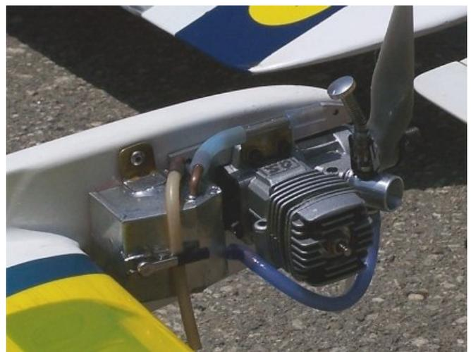
Dave Hulls' Clown is neat as a pin! Engine is an OS CVA .15 aero R/C conversion. The RC carb has been replaced with what appears to be an older OS Max venturi & needle valve.
