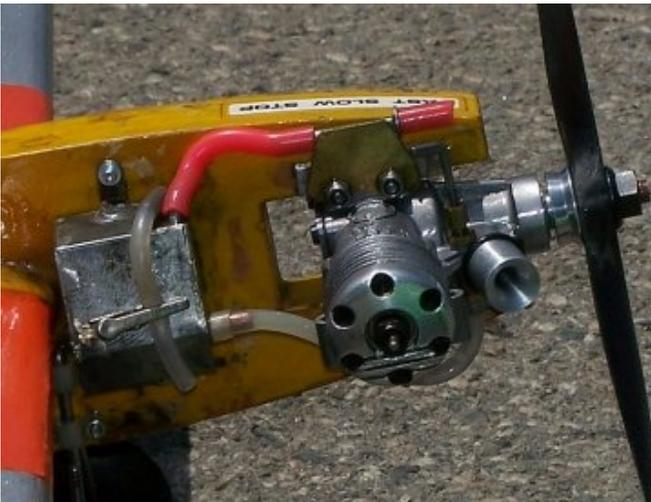
Kevin Kusiks' model takes the basic approach. Not much to maintain or go wrong here. The motor is a Supertigre G15-.19 with home made venturi. No shutoff, with this tank setup it would be difficult to fit one in. Note the fuel filler tube is soldered to a
