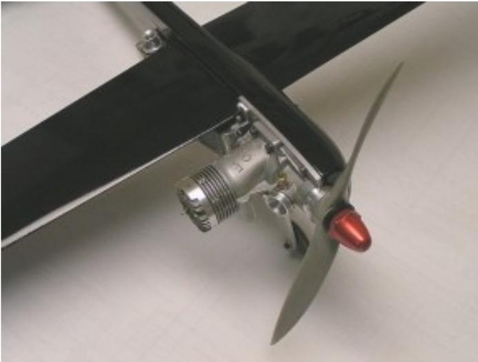
Here are some pics of my TQR's, the black one is my own design and is powered by an O.S. 40H. and uses a Mezjlik shutoff. The other is a Matson Scorpion, and uses a Garner K&B .40 with an exhaust prime and a Dave McDonald shutoff. Both fly great and are very reliable on the restart.
