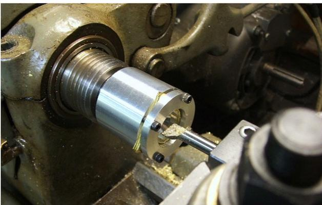
the shim stack as shown in the above photo. The ID of the fixture is the same size as the shim ID. Remove the shim stack from the ID fixture and load them on the OD fixture. Make sure the stack is compressed well when tightening the end cap screw.
