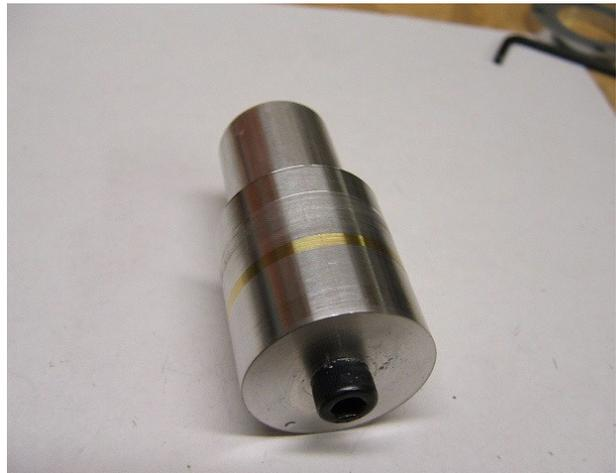
(above photo) if you don't get in a hurry and cause the stack to slip. The last photo shows the completed shims as they are removed from the OD fixture.
