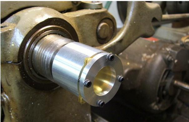
The second photo shows the shim material loaded in the ID fixture with the fixture mounted in the lathe. I drill a hole in the center of the stack then use a boring bar to cut the ID of
