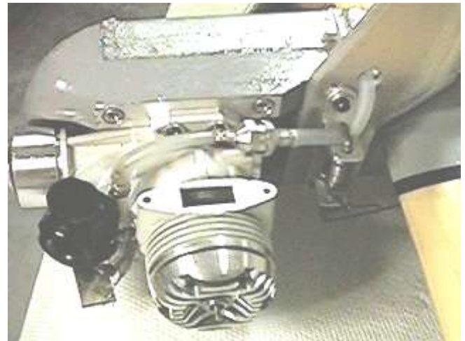
Detail from below. Note position of shutoff & fuel pickup line from tank, passes through hole in landing gear strut.
