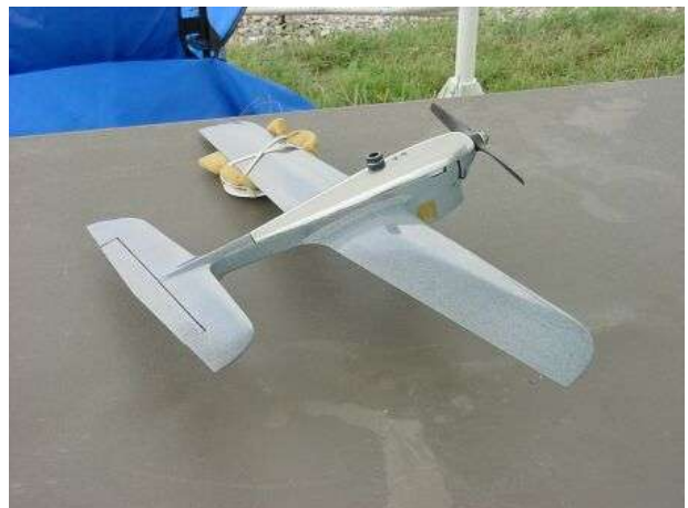
Mike MacCarthy sent me a few more details on his plane. It is a 75% Gillott Shark, Tatone pan, Nelson .15 with NO minpipe.
