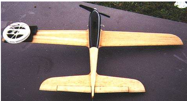
Bob Kerr's Hamster. 75% scaled Gillott Shark. Motor is a NovaRossi .15 Car motor reworked by Tim Gillott.
