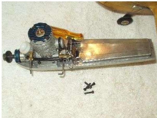
Motor crutch detail. NovaRossi power. Note that tank is silicon'd into the crutch along with shutoff. Don't ask why there's 2 needle valves! Using his own crutch, Bob was able to create some additional space.
