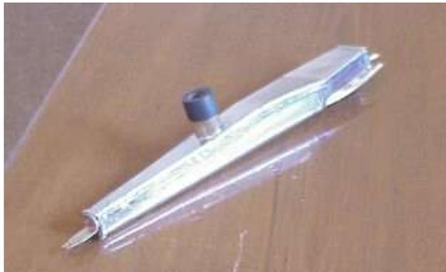
Tim Stone's Hamster tank. Pressure line ends in filler neck, fuel pickup at edge of tank angle. Shape determined by pressing clay into pan cavity & making patterns from the clay plug. 2.5 OZ is about as much as you can get in a DARP pan. Runs are very consistent with this setup & no check valve is required on pressure line.
