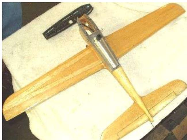
Top view shows tank placement. Much more room for fuel tank than with a typical upright. Tank looks to be around 3 OZ.
