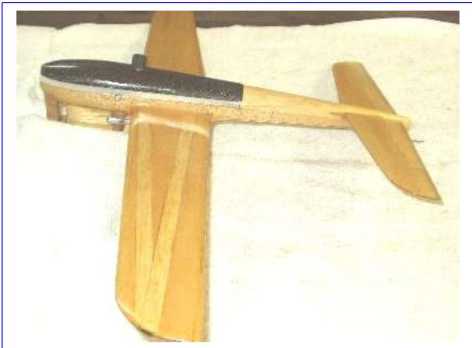
Bob Kerr's Hamster. Bob has taken an all-out approach to this event and built one of the nicest Rats to hit the circle. Bob's rodent has a carbon fibre custom molded top shell, and motor crutch made from 1/4" aluminum plate.
