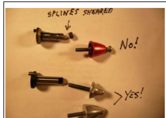
A 5-40 TPI prop stud (screwed ALL the way in) & spinner is used to prevent the Killer Bee/Venom type crankshafts from shearing at the splines.
