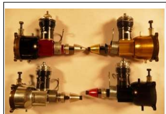
Cox .049 mouse racing engine variants: Top L-R: Venomw/ Galbreath head & Golden Bee. Bottom L-R: Silver Bee & Black Widow.
