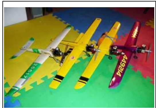
Paul Gibeault's all Cox .049 powered Streaker mouse racing fleet ready to race.
